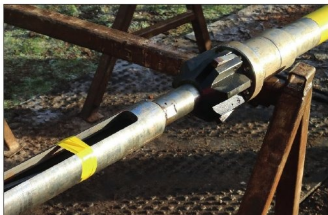
The S Geobor wireline high pressure dilatometer system
